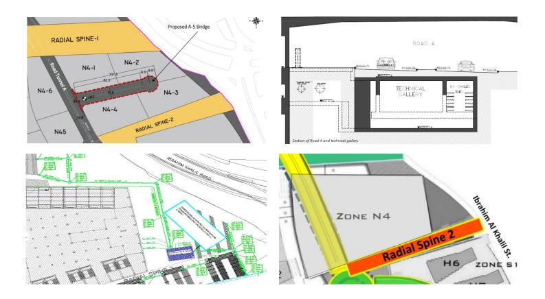
Due to cancelation of Mussalah building, a Radial Spine (2) is designed to allow access to N4-3 and N4-4 areas. Also, the storm water storage is located in N4-3 area to collect storm water from Radial Spine 1 and Radial Spine 2. Water collection is done by shifting the tanks, manholes, and pipes' networks out of N4 area.
