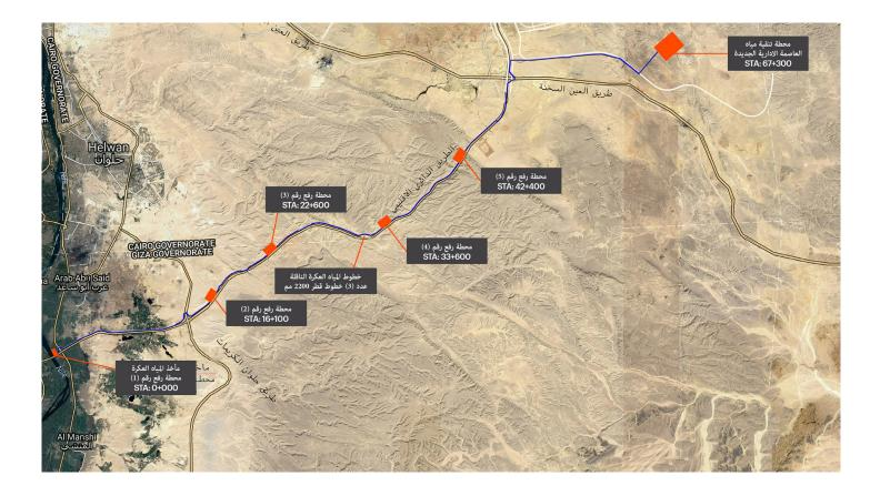
ECG scope in terms of piping works covers hydraulic calculations, hydraulic profile, study of hydraulic balance of the pipeline, strategic ground tanks, and transmission pipelines & crossing with canals, drains & roads. Additionally, water hammer analysis is administered to protect the pipeline from hammer impact. ECG scope in terms of booster-pump station works covers hydraulic calculations, plant layout, piping & instrumentation diagram (P&ID), and plant mechanical general arrangements.
